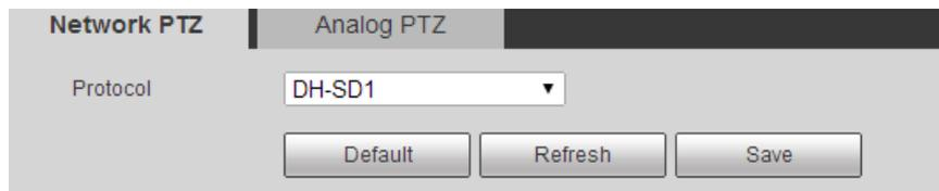
The screenshot shows a web interface for configuring PTZ settings. At the top, there are two tabs: "Network PTZ" (which is active) and "Analog PTZ". Below the tabs, there is a "Protocol" label followed by a dropdown menu currently set to "DH-SD1". At the bottom of the interface, there are three buttons: "Default", "Refresh", and "Save".
